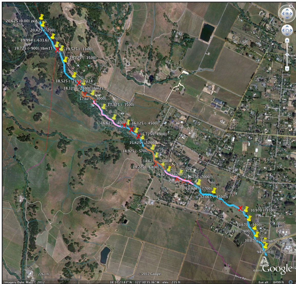
Figure 44. Estimates of distance station locations are shown at the yellow pinpoints along the mainstem Carriger Creek, which is shown as a thick blue line. The first sets of numbers are the distance stations in feet that are based upon zero being located at the confluence of Felder Creek. The numbers in parentheses are the stations established during the field survey with zero being located upstream of the Grove Street box culvert. As also indicated in Figure 45, the light brown lines represent the reaches that have had significant incision since WY 2006, while the light pink lines represent reaches with significant deposition. Several braided segments exist along the mainstem but they have not been mapped. The direction of flow is from top to bottom of the picture. Red X's represent approximate locations of inflection points where there are significant changes in stream gradient.
